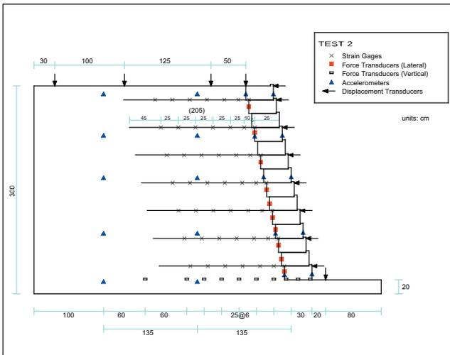
*Test Two* was built in exactly the same manner as Test One, with the only change found in the grid spacing. The objective was to provide an accurate assessment of the influence of spacing on SRW design. Using the same embedment length, grid layers were placed on every other course of block.
