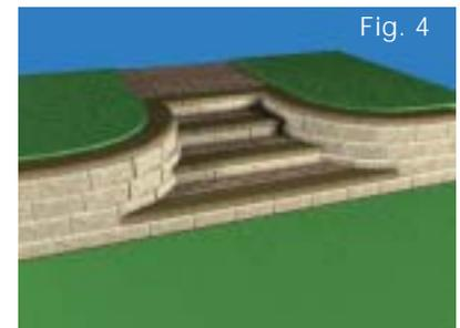
Finish stair treads using AB Capstone, landscape pavers or flagstone. Adhesive is recommended on tread material to secure in place.
